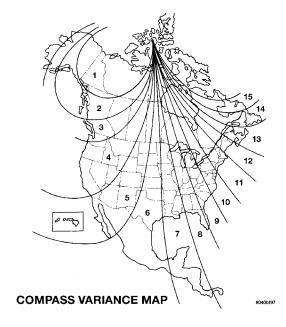
To set the variance: Turn the ignition ON and set the display to "Compass/Temperature." Press and hold the RESET button approximately five seconds. The last variance zone number will be displayed. Press the STEP button to select the new variance zone and press the RESET button to resume normal operation.
